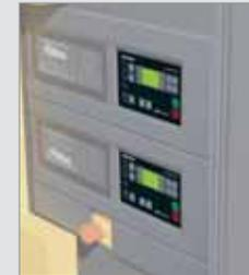
Operational status can be determined at a glance at the plain text display (many language options). Standard communication interface and Profibus DP enable remote monitoring and integration with Sigma Air Manager and plant controls.
