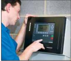
be adapted to almost any system and manage up to 16 compressors, blowers, or vacuum pumps. It also manages dryers, filters and drains. SAM balances service hours, prevents simultaneous motor starts and maintains tight pressure control – something standard sequencers cannot do!
